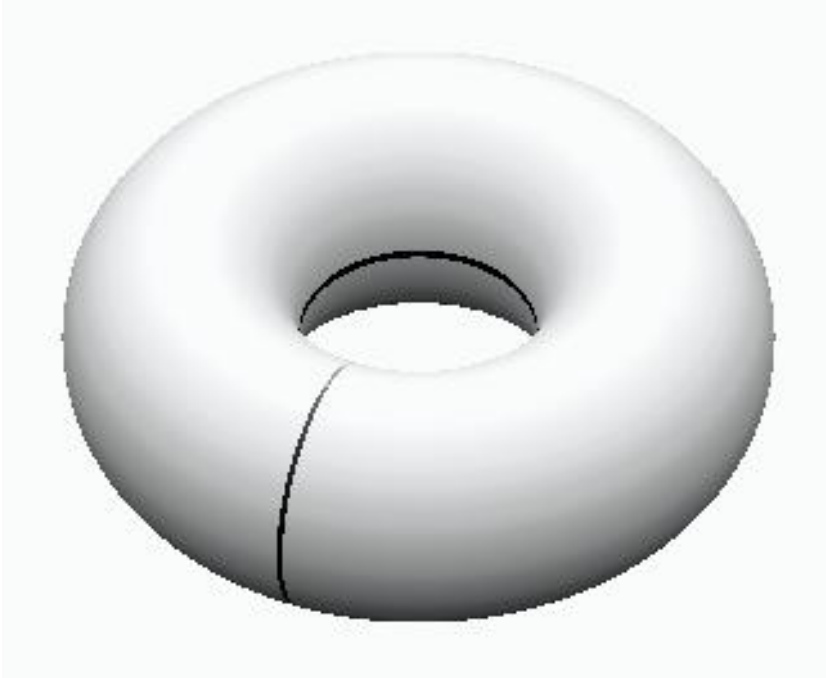
Figure 26. Torroidal topology of computational domain that is periodic in both directions. Gaps in torus illustrate how the domain wraps around on itself.
